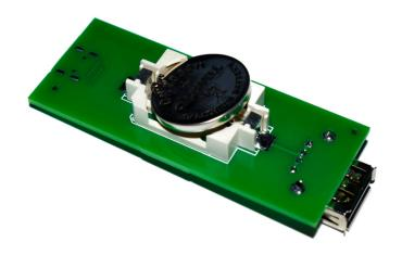
**Step 3:** Firmly press down on the battery until it snaps into place.
