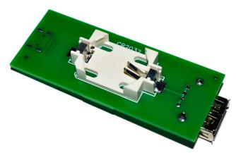
**Step 2:** With the positive side of the battery facing up insert one edge of the battery under the metal fingers of the holder.
