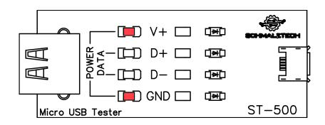
Broken wire. A single wire inside your cable has broken. Cables that test like this should be replaced.
